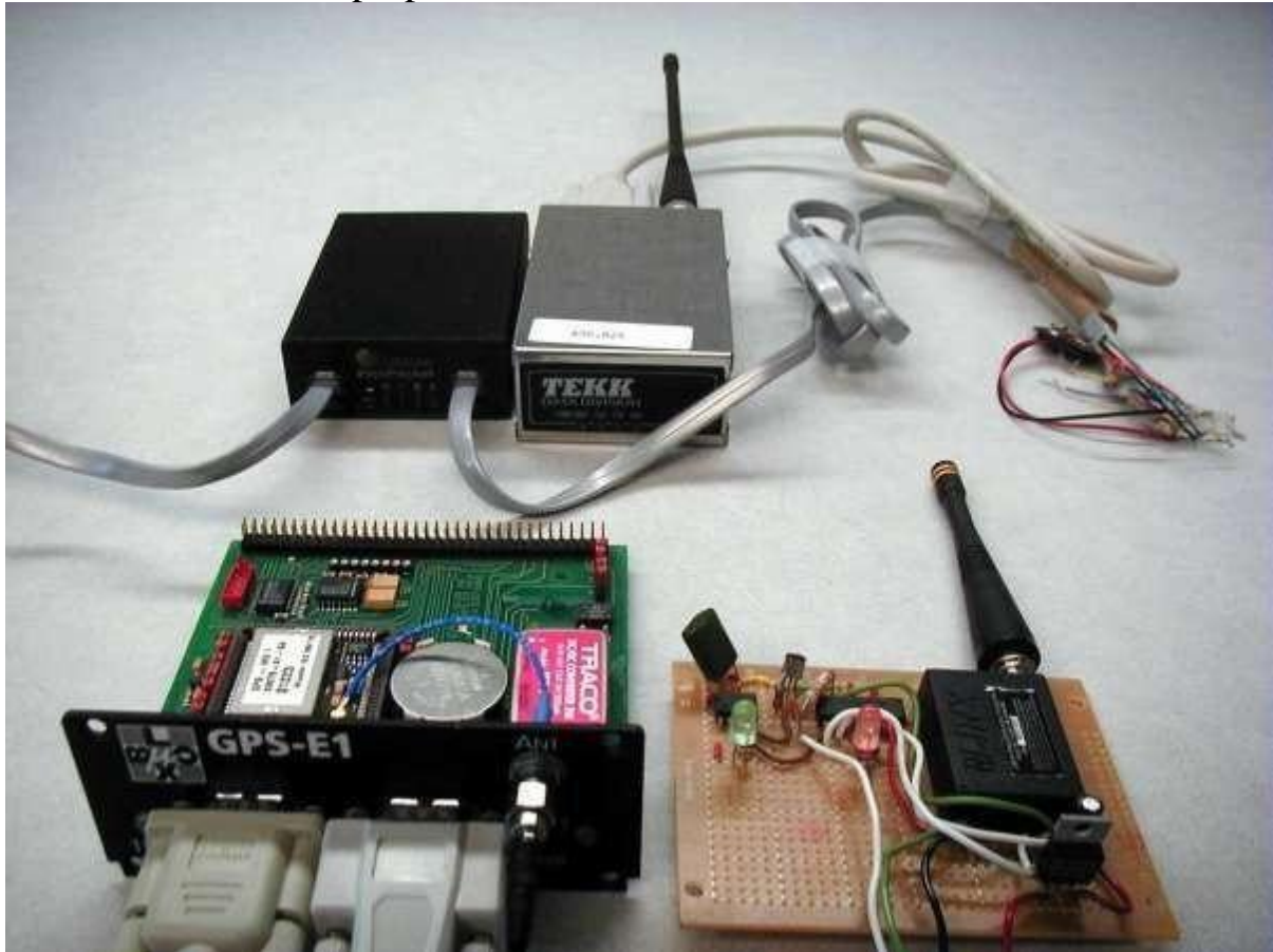
(Typical Hardware of the Wireless Sensor Networks connected with the GPS)
